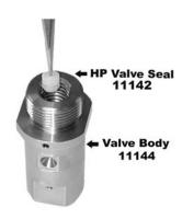
Push the Seal into the Valve Body with the Seal Tool. Load the Seal Back-up Ring into the Valve Body behind the Seal and push down until the Back-Up Ring is flush to the top of the bore. Screw the Valve Screw-11218(Not part of the Insta 1 On/Off Valve Kit) into the Valve Body until it bottoms out.
