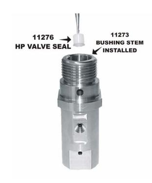
Push the Seal into the Valve Body using the Seal Tool. Place the Backup Ring concave end down onto the Seal and push down until the back of the Ring is flush with the bottom face of the bore.
