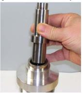
**9.** Use the blunt (non-stepped) end of the installation tool to hand press the seal the rest of the way into the cylinder.
